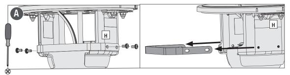
Remove any existing bracket prior to installation. Only use the provided Hunter ceiling bracket that came in your fan's box.
