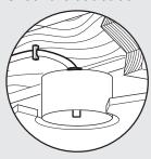
You must be able to secure the fan to building structure or fan-rated outlet box and clearly marked acceptable for fan support of 70 lbs (31.8 kg) or less.
